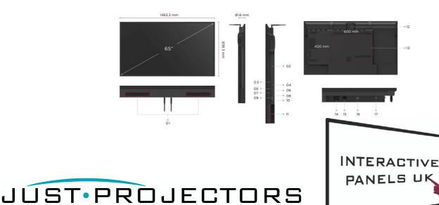
1. Speaker 2. OPS Slot 3. USB 2.0 4. RS-232 5. USB 3.0 6. USB-C 7. HDMI 1(ARC) 8. HDMI 2 9. HDMI OUT 10. HDMI 3 11. Control Panel 12. WiFi Slot 13. VESA® Wall Mount (600x400mm)
